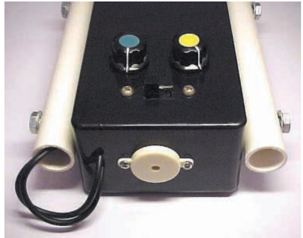
Case mounted between the conduit handle and search head shaft.
