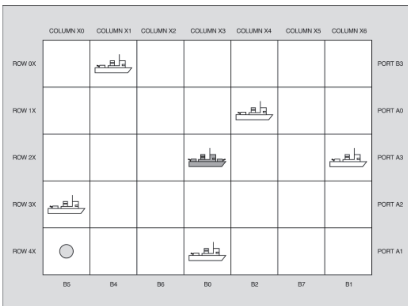
Fig.1. How the ships are positioned. The enemy battleship at the centre of the display is unseen. The circle represents your battleship and is a "moveable" flashing l.e.d.
